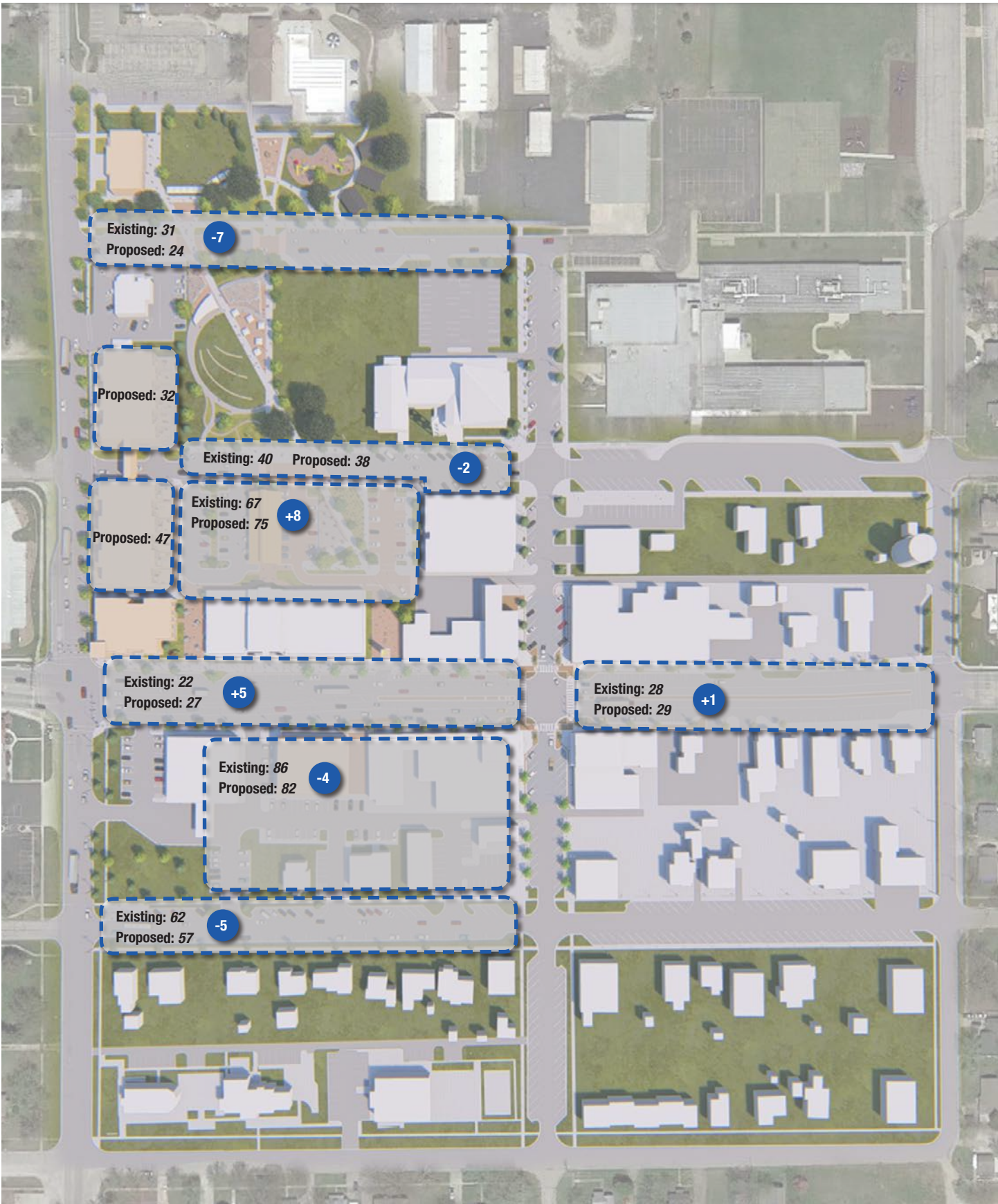
Figure XV - Parking Inventory. Streets and lots not called out on this plan, indicate no changes in quantity of parking stalls.
