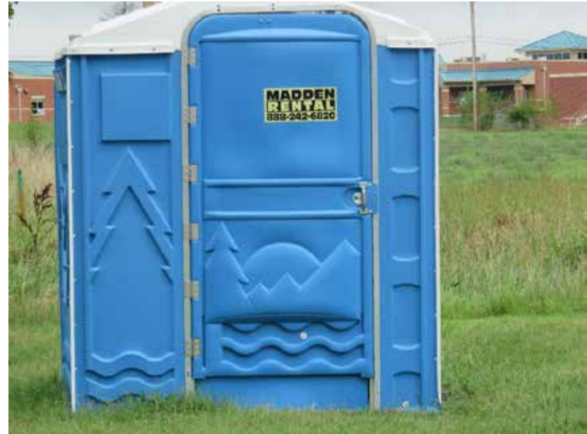
Accessible portable toilet room should be on accessible route
