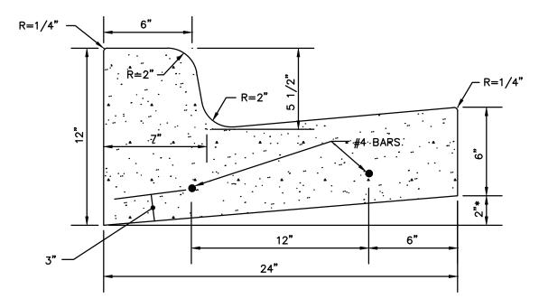
\* FOR 8" ASPHALT PAVEMENT, CONCRETE FACE OF CURB SHALL BE 7\frac{1}{2}".
