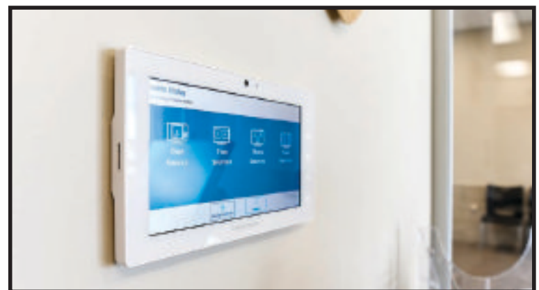
The lobby is controlled via a wall-mounted Crestron touchpanel.
