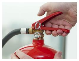
the nozzle pointing away from you, and release the locking mechanism.
